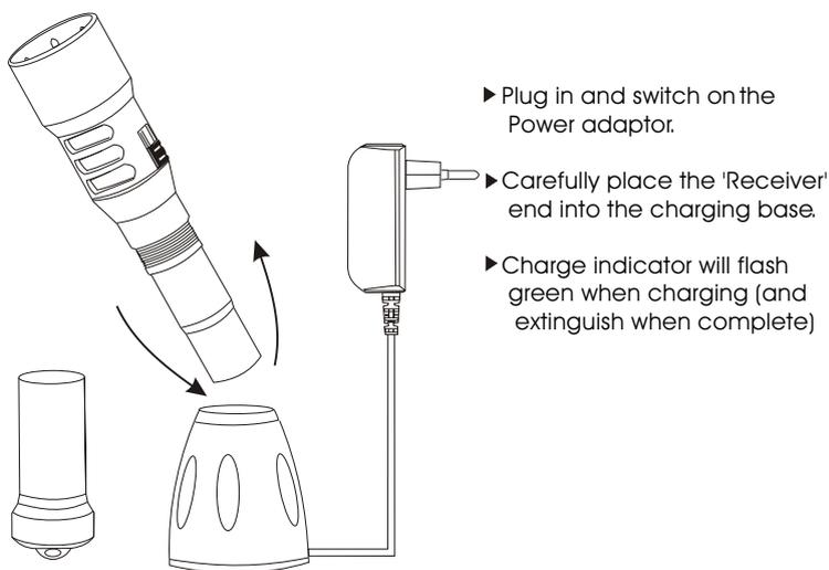
► Plug in and switch on the Power adaptor.
